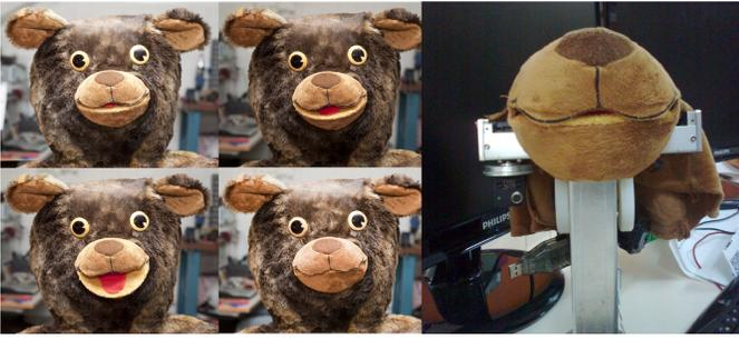
Fig. 4. In the left hand side it can be seen the robotic mouth mounted on the Ursus 2 robot. In the right hand side it can be seen the mouth system separated from the rest of the robot, as used in section VI.
